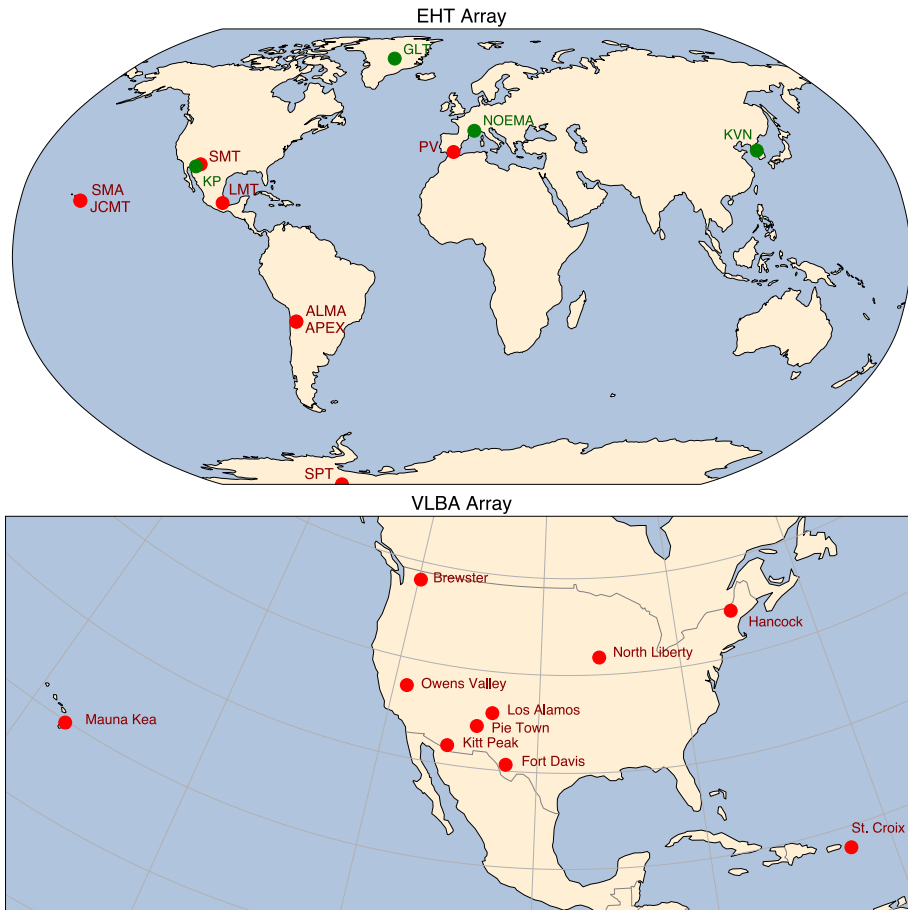
Figure 2.3: VLBI arrays. Locations of the antennas in the EHT array (top) and the VLBA array (bottom). For the EHT array, red points mark the antennas present in 2017, while green points denote antennas added between 2018 and 2025.
